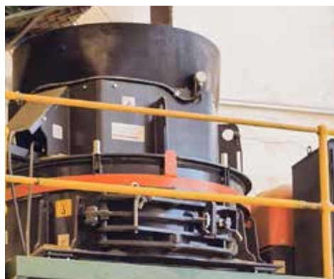
The VSI crusher from Sandvik is central to the Enviro Sand waste glass management process.
