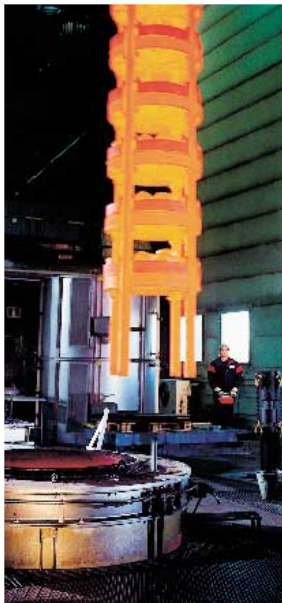
At the Sandviken plant, several investments in increased capacity and productivity were made in 1999 – for instance, a new bell furnace for annealing of strip steel.
